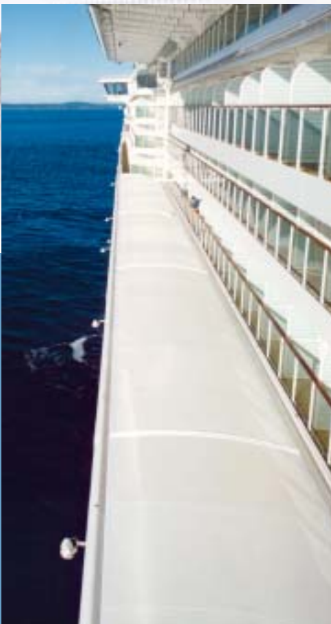
Radiance of the Seas, ©* Liveboat covers (approx. 980m 2 ) Abdeckung der Rettungsboote (ca. 980m 2 )
